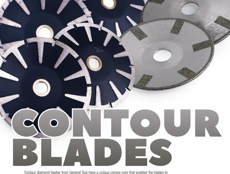
Contour diamond blades from General Tool have a unique convex core that enables the blades to cut perfect circles and curves. These tools are ideal for cutting sink openings and arcs with grinders and handsaws. We manufacture three different contour blades with fine diamonds not only on the rim, but also on the core which help prevent the blade from binding and undercutting. Each blade is made with cutting-edge engineering and materials of supreme quality for both speed and longevity.
